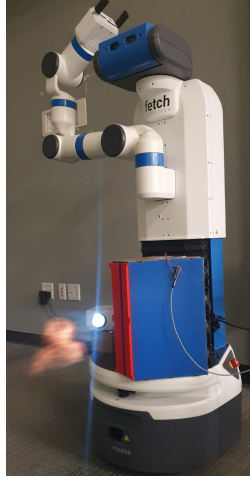
Figure 1: The working prototype of the implemented fog screen device and a projector placed on the base of a Fetch robot. The projected content is a red human icon, which is useful in search-and-rescue scenes to indicate the sign of life of a human victim. It is one of the use cases where no suitable flat surface exists for the robot to project to communicate with humans.
